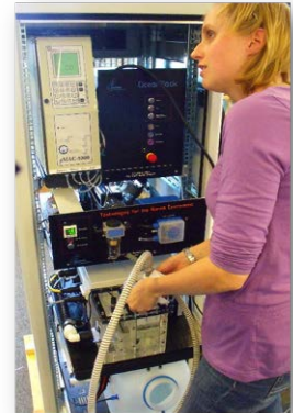
Photo: complete nutrient and pCO 2 analyzing system for AquaCulture applications
